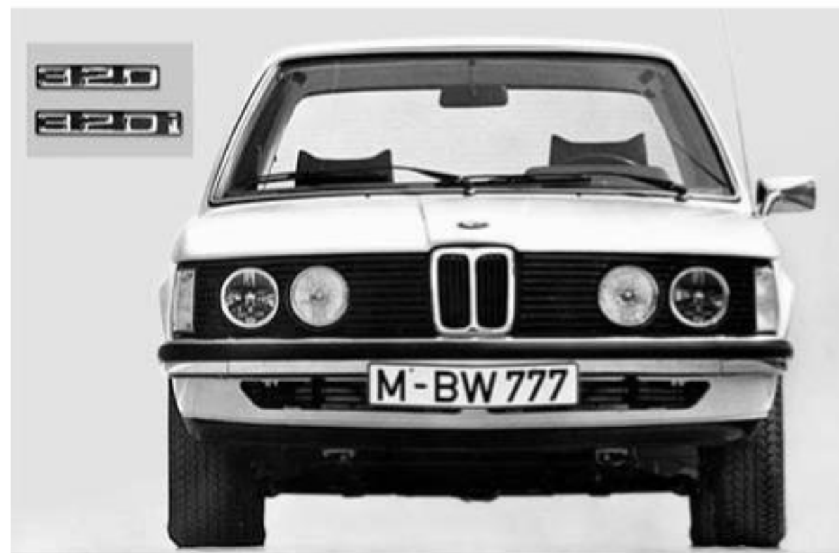
Vier Scheinwerfer blieben den 2-Liter-Modellen vorbehalten. Four headlamps were reserved for the 2-litre models.
