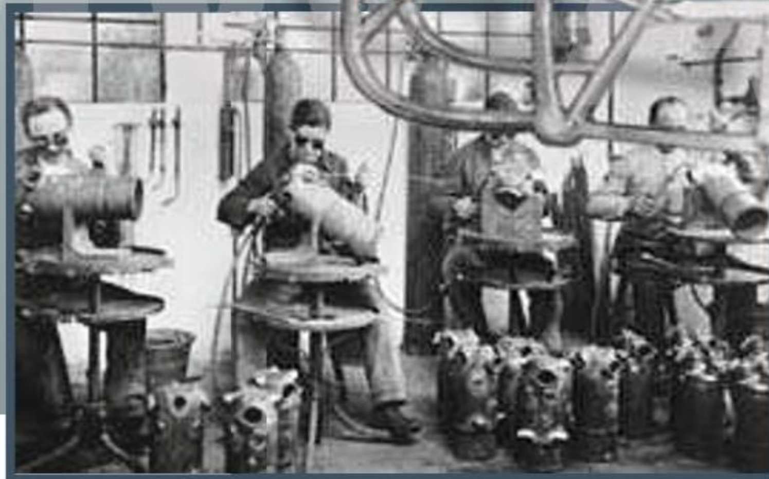
← LEFT Competence from the very outset: precision-grinding of lightweight cast parts right after World War II (right) and in the Fifties (left).
