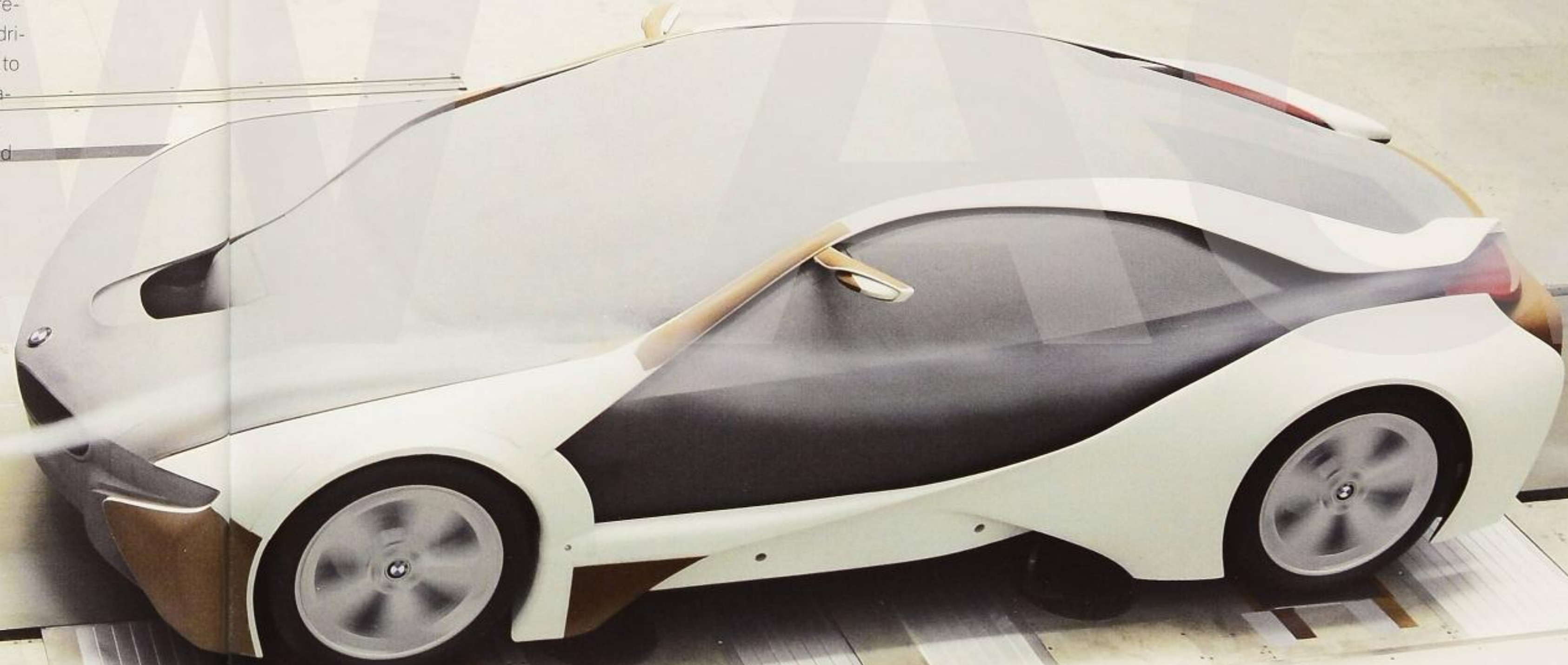
↓ BELOW The new Aerodynamic Test Center (AVZ), built in 2009 in the north of Munich, strengthened the development of aerodynamics, which is a major cornerstone of BMW's EfficientDynamics. Here you can see the sports car study BMW Vision EfficientDynamics in the wind tunnel of the AVZ.
