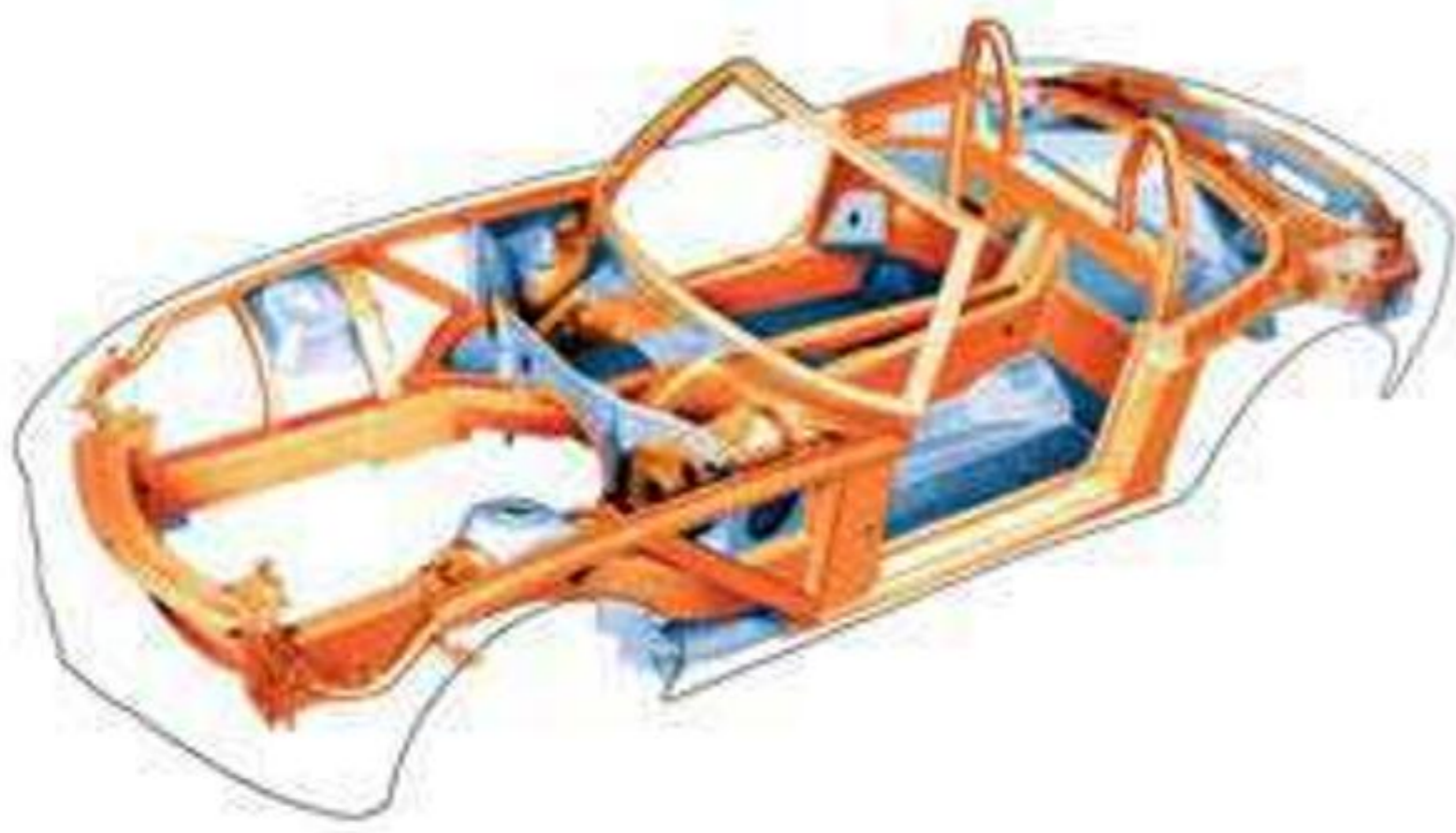
← LEFT The aluminium space frame construction of the BMW Z8 saves a lot of weight.
