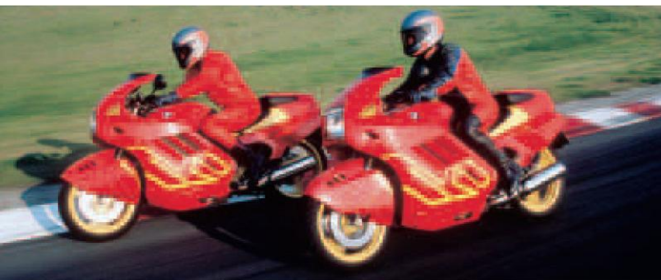
Four-valve super sports models with 100 bhp, avant-garde full fairing and refined aerodynamics: BMW K1 from 1990.
